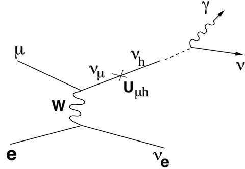
FIG. 1: Schematic illustration of the production and subsequent radiative decay of heavy neutrino in the ordinary muon decay.
