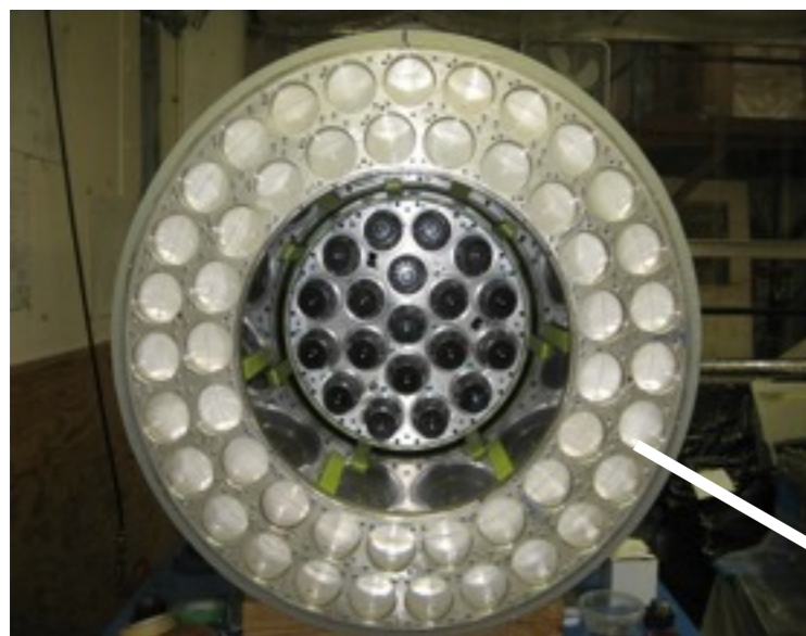
Monolithic NaI(Tl) crystal surrounded by 97 pure CsI crystals
