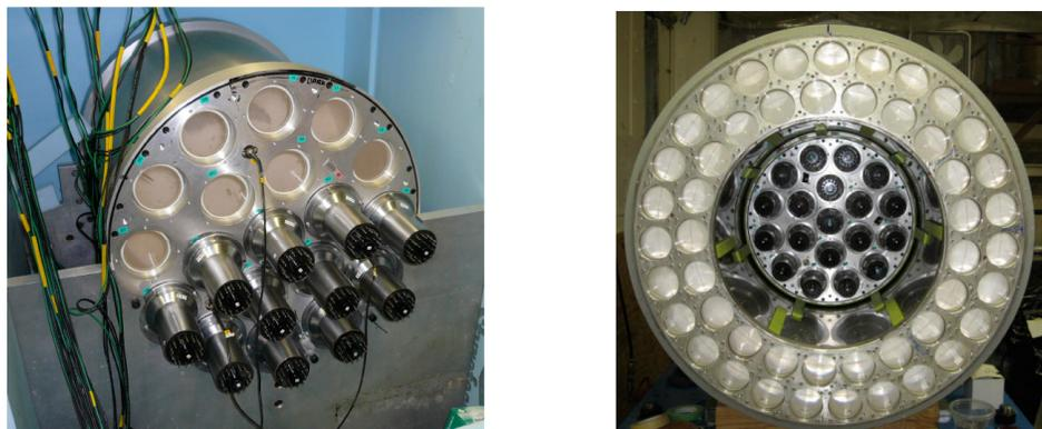
Figure 3.10: (Left) Back side of the NaI(Tl) crystal on the test bench. (Right) The NaI(Tl) crystal and the 97 CsI crystals while the calorimeter was under construction [9].
