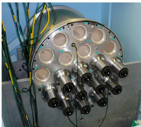
Figure 3.13: View of the NaI crystal from the back side on the test bench.
