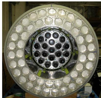
Figure 3.14: The NaI crystal surrounded by the 97 crystals of CsI arranged in two layers.
