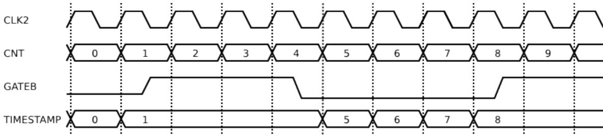
Figure 4.9: Timing chart of the time stamp. The time stamp (TIMESTAMP) buffers the number of counter at the gate (GATEB) closing.
