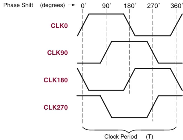
Figure 3.11: Quadrant Phase Shift Outputs Shift CLKIN, Each by a Quarter Period
