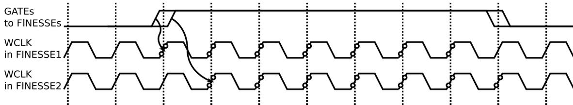
Figure 2.9: Diagram to determine the write enable (WEN) region by a gate signal (GATE). The data acquisition region could slip by 8ns because of 125 MHz operation clock (FPGA CLK) and WEN is created from GATE by FPGA CLK. The GATE timing cause different data acquisition regions by two point corresponding with 8 ns. This means each triggers' waveform can have different time offset without adjusting the timing between GATE and CLK.
