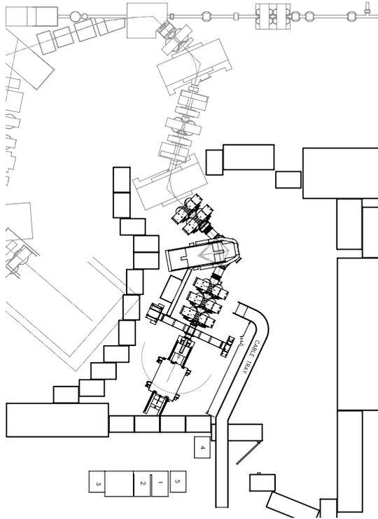
Figure 1.5: Schematics of M13 beam line. The black line shows reachable area.
