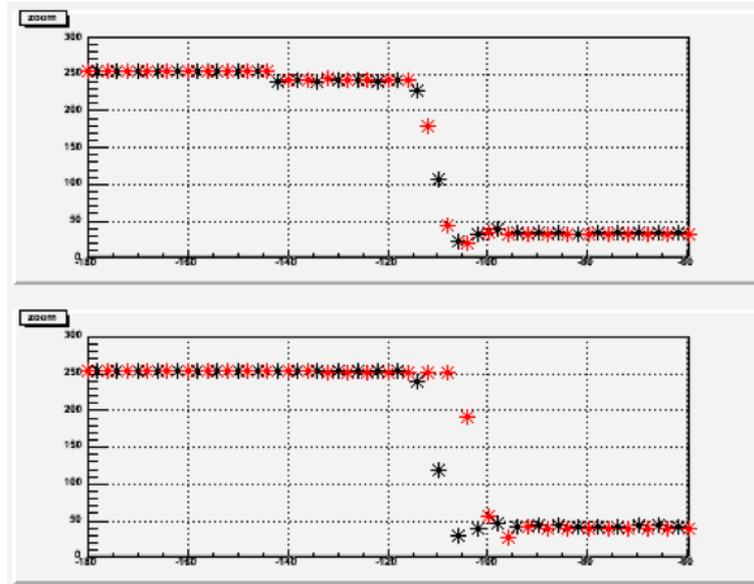
Figure 3.1: Waveform with time offset shift between two ADCs. Black points are the samples from one ADC, and Red points are the samples from another ADC. One ADC is shifted by two points (8 ns) because the data is sent by 125 MHz from ADCs to FIFOs.
