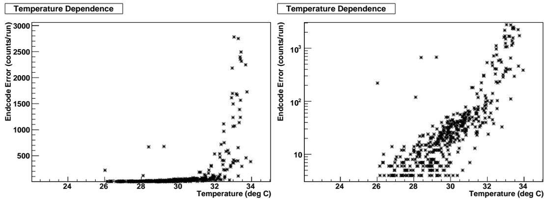
Figure 3.5: Endcode Error versus Temperature in the electronics rack. A strong correlation between endcode error and temperature exists.
