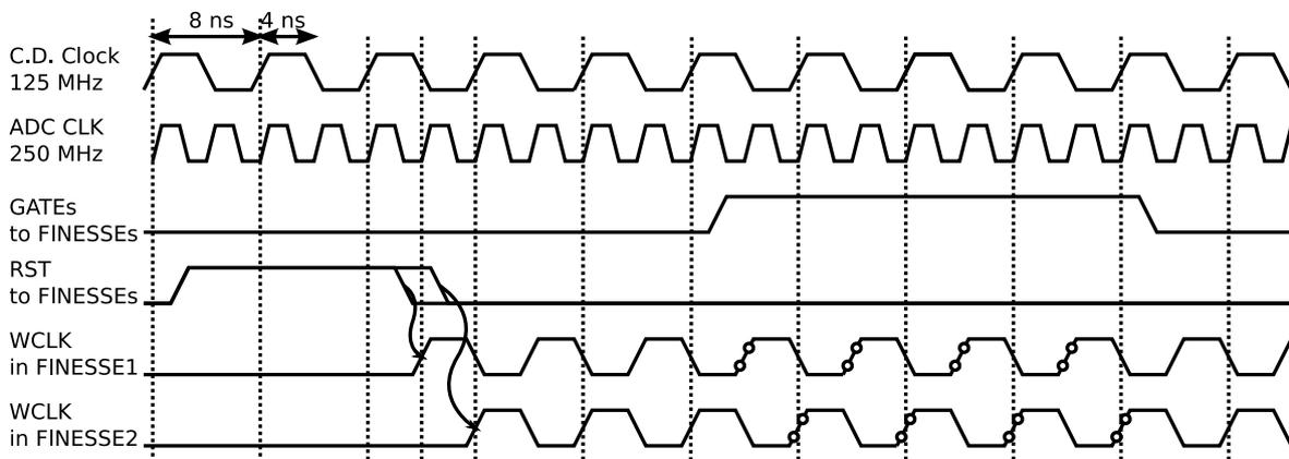
Figure 2.10: Diagram to determine the phase of 125 MHz write clock (WCLK) from ADCs to FIFOs by reset (RST). CD distributes 250 MHz clock (CLK) and 125 MHz latched RST. ADC divide the CLK to 125 MHz WCLK by RST timing. The two phases cause different data acquisition regions with same latched gate (GATE) by one point corresponding with 4 ns. This means two FINESSEs or two runs can have difference without adjusting the timing between GATE and CLK.
