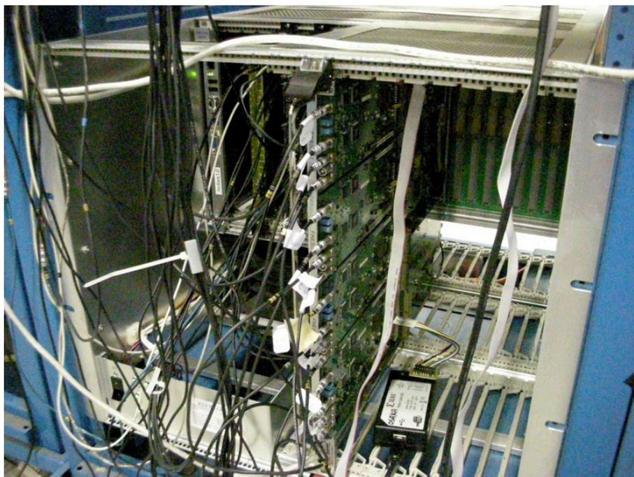
Figure 2.4: KEK-VME with the COPPER board
