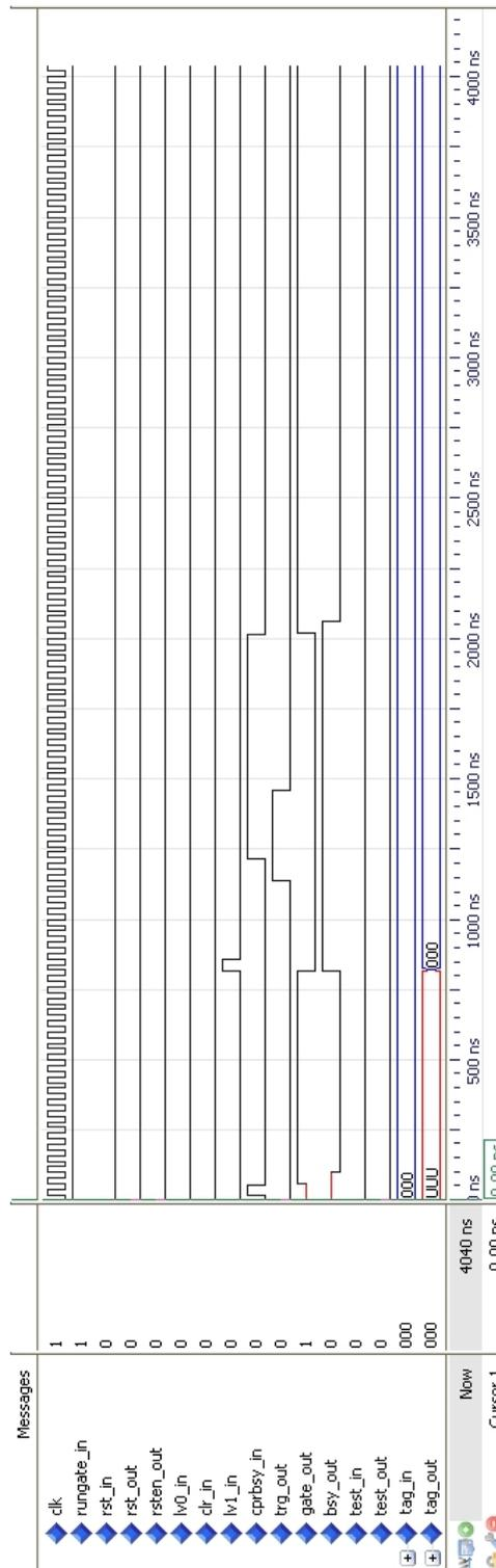
Figure 4.4: Level 1 trigger. This trigger is same with the previous one. level 1 trigger (LV1\_IN) stops the gate (GATE\_OUT) and starts the busy (BSY\_OUT), and sends the trigger for COPPER (TRG\_OUT) after a few hundred ns. And then the closing timing of busy (CPRBSY\_IN) starts GATE\_OUT and stops BSY\_OUT, respectively.
