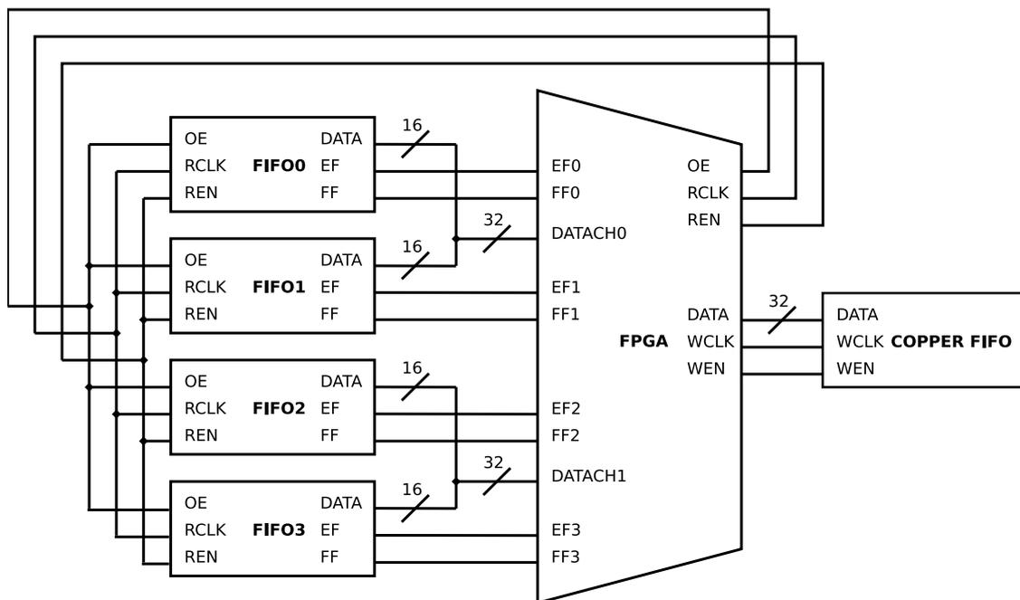
Figure 3.3: Diagram to read and write the data from FINESSSE FIFOs to COPPER FIFOs. The empty flags create the endcode.
