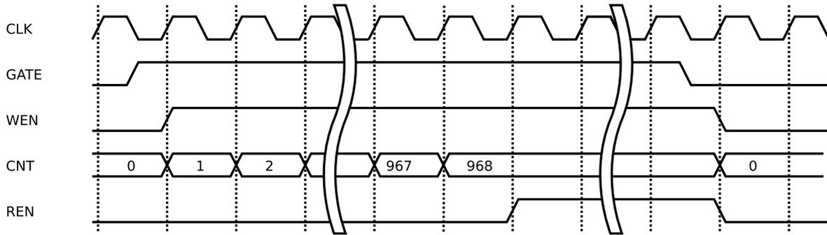
Figure 3.16: Logic diagram to buffer the data. Counter (CNT) starts to count clock signal (CLK) at the gate coming, and Read enable (REN) starts to dump the data when CNT becomes 968 corresponding with 7.7 us.
