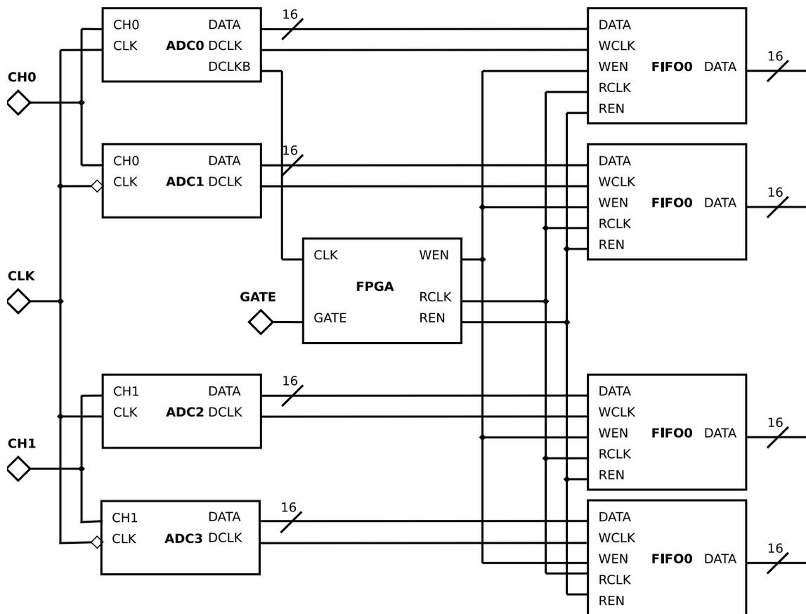
Figure 3.15: Diagram to send and dump the data. The FPGAs on each FINESSES control the signals, and FIFOs buffer the data for 7.7  $\mu$ s.
