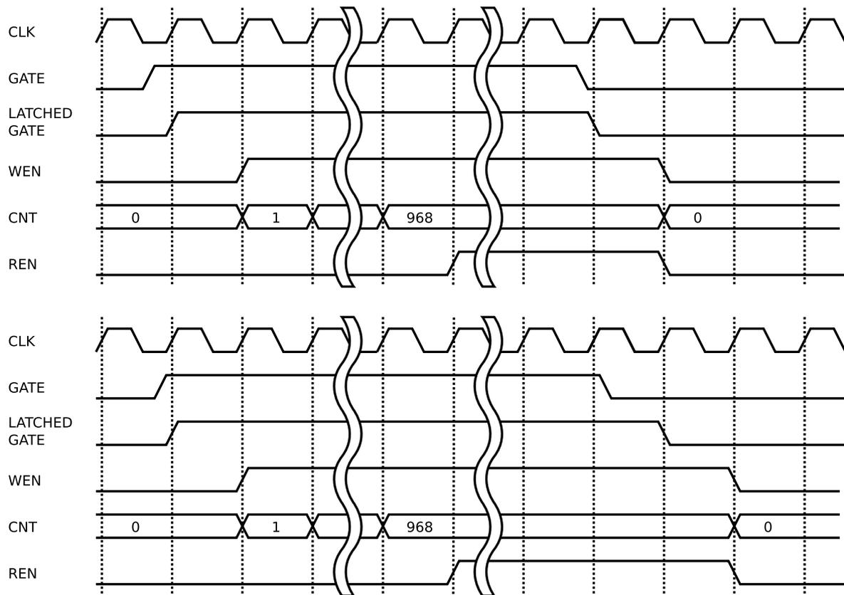
Figure 3.21: Timing chart of gate (GATE), write enable (WEN), and read enable (REN) with latched GATEs. The latched gate makes a WEN and the counter (CNT) which makes REN. The difference between WEN and REN lengths is the data length.
