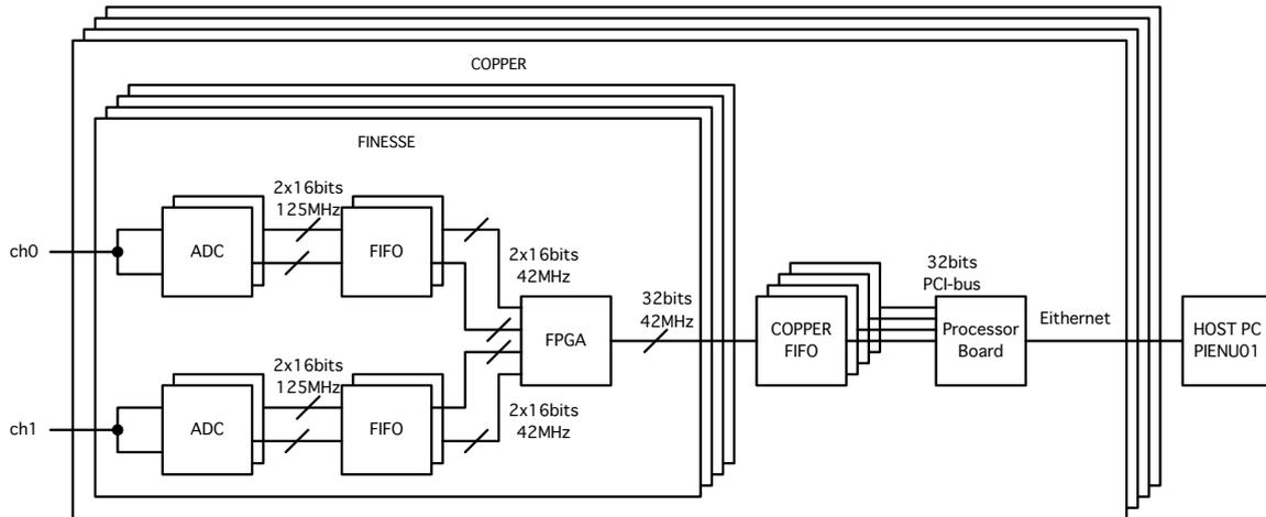
Figure 2.3: Schematic diagram of the data flow in FINESSE 500-MHz FADC.
