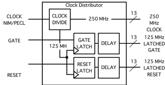
Figure 2.5: Schematic diagram of Clock Distributor.
