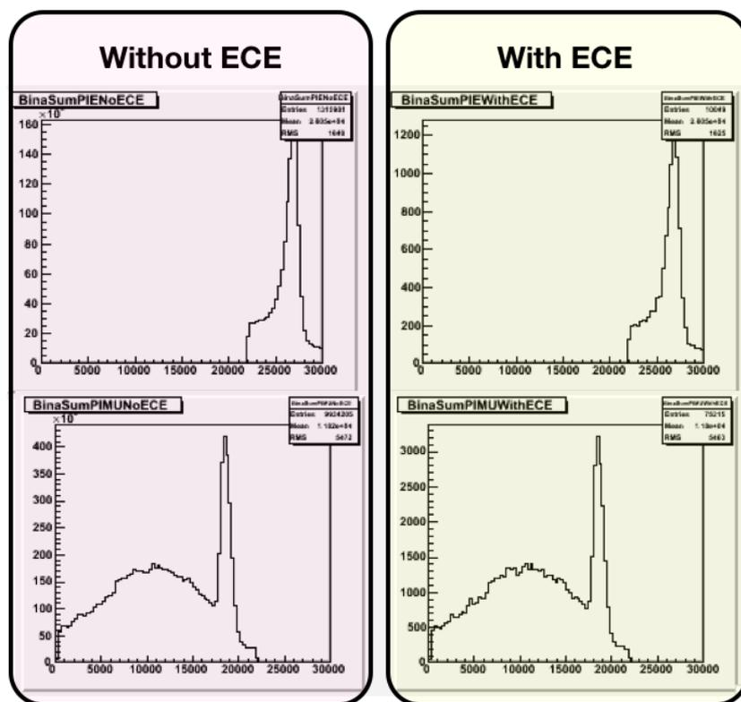
Figure 3.7: Positron energy spectra in NaI with and without endcode errors. Left and right histograms are without and with endcode error, respectively. Upper and down histograms mainly consists of  $\pi \rightarrow e$  and  $\pi \rightarrow \mu \rightarrow e$  decay positrons, respectively.
