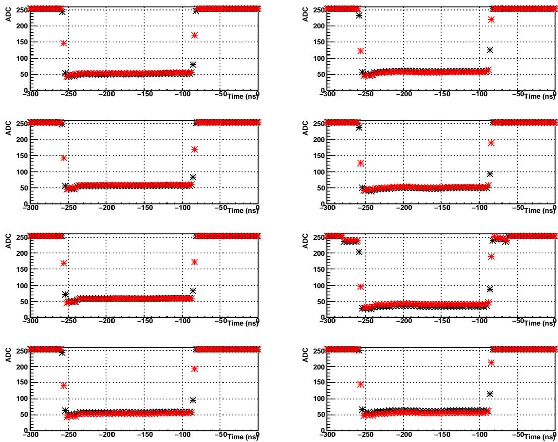
Figure 2.12: The waveforms of the synchronous signals. The synchronization of signals is checked by the timing just over the threshold.
