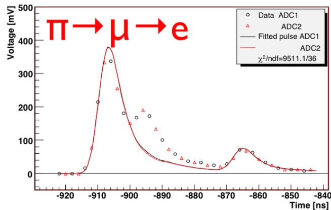
Figure 1.8: Typical wave form in the target
