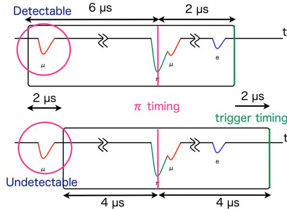
Figure 4.1: Schematic diagram of the trigger delay by TIGC.
