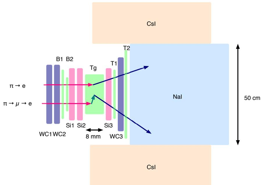
Figure 1.3: Schematics of the PIENU detector
