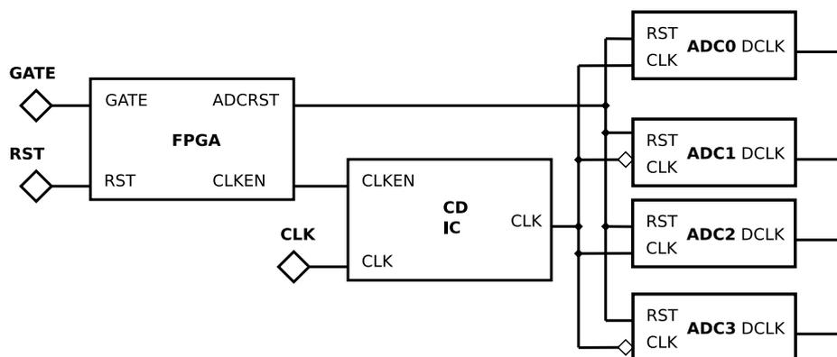
Figure 3.22: Diagram to reset the ADCs & Clocks.
