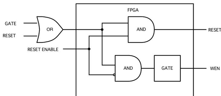
Figure 3.25: Diagram of select gate or reset from FINESSE input. Reset signals initialize the internal 125 MHz clocks, and gate signals make write enable signals to FIFO. Reset enable signal select gate or reset by logical AND in FPGA.
