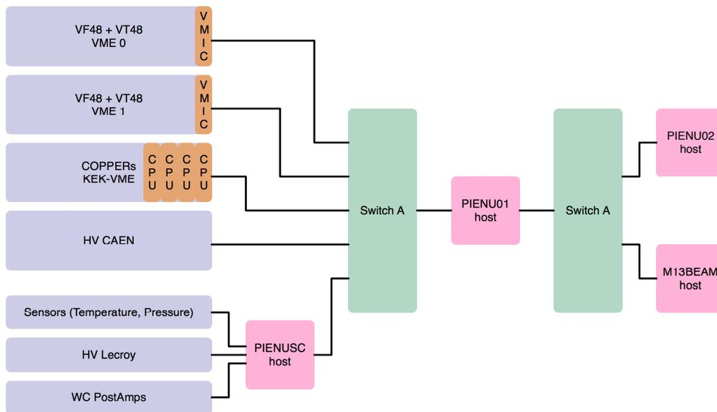
Figure 4.8: Schematics of DAQ network.
