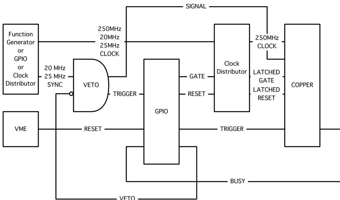
Figure 2.11: Logic diagram to make the synchronous signals. Function generator, GPIO, or Clock Distributor send the signals and the clock synchronized with each other. The signals, gates and resets into COPPER are synchronous because the clock synchronized with the signals creates the CD clocks, latched gates and resets.
