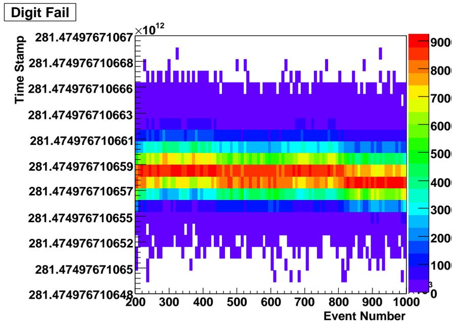
Figure 4.13: Event ID versus Timestamp. The timestamps at carrying the digit is studied. The triggers after each resets caused the almost same timestamp. 281474976710655 is 0x ffff ffff ffff. 281474976710656 is 0x 1 0000 0000 0000. In the out of Y axis, there are no event.
