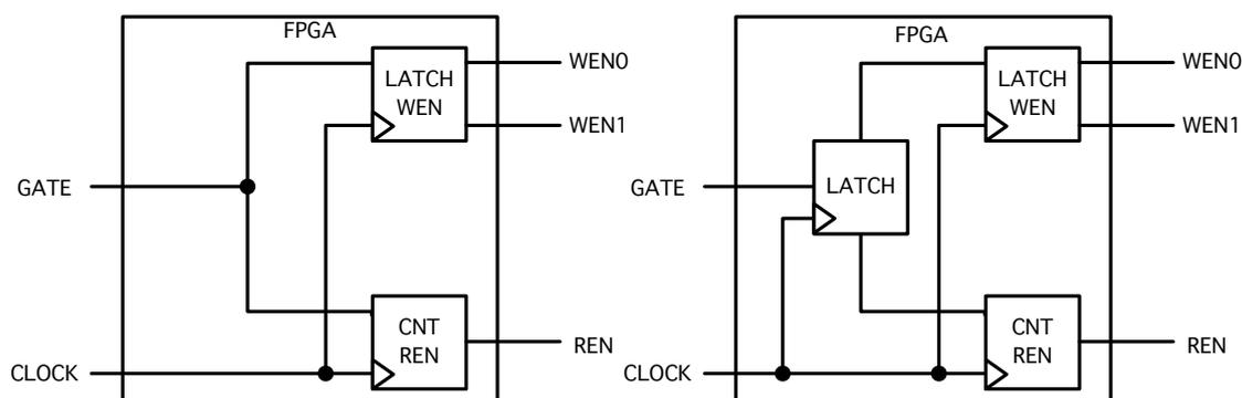
Figure 3.20: left: Diagram of a gate signal (GATE) distribution in FPGA. GATE is distributed to the modules to make write enable (WEN) and read enable signals (REN). right: Diagram of a latched gate signal (latched GATE) distribution in FPGA. The GATE is latched and then distributed to the modules to make write enable (WEN) and read enable signals (REN).
