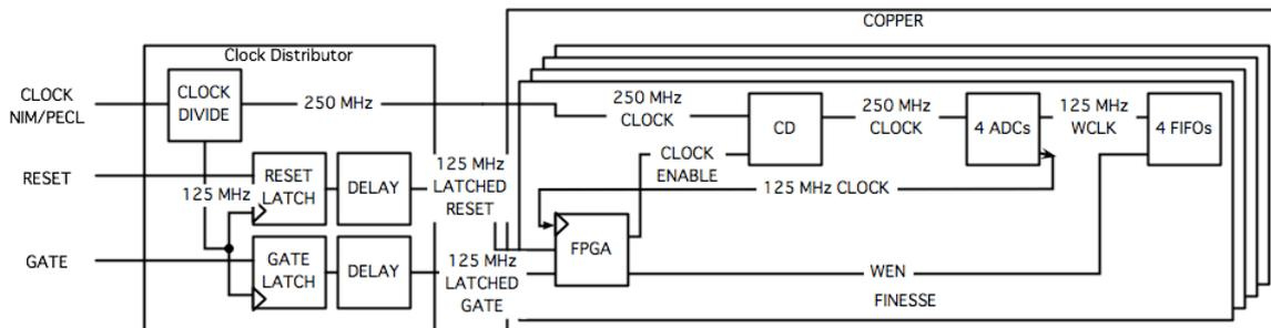
Figure 2.8: Diagram of connections between CD and COPPER to synchronize.
