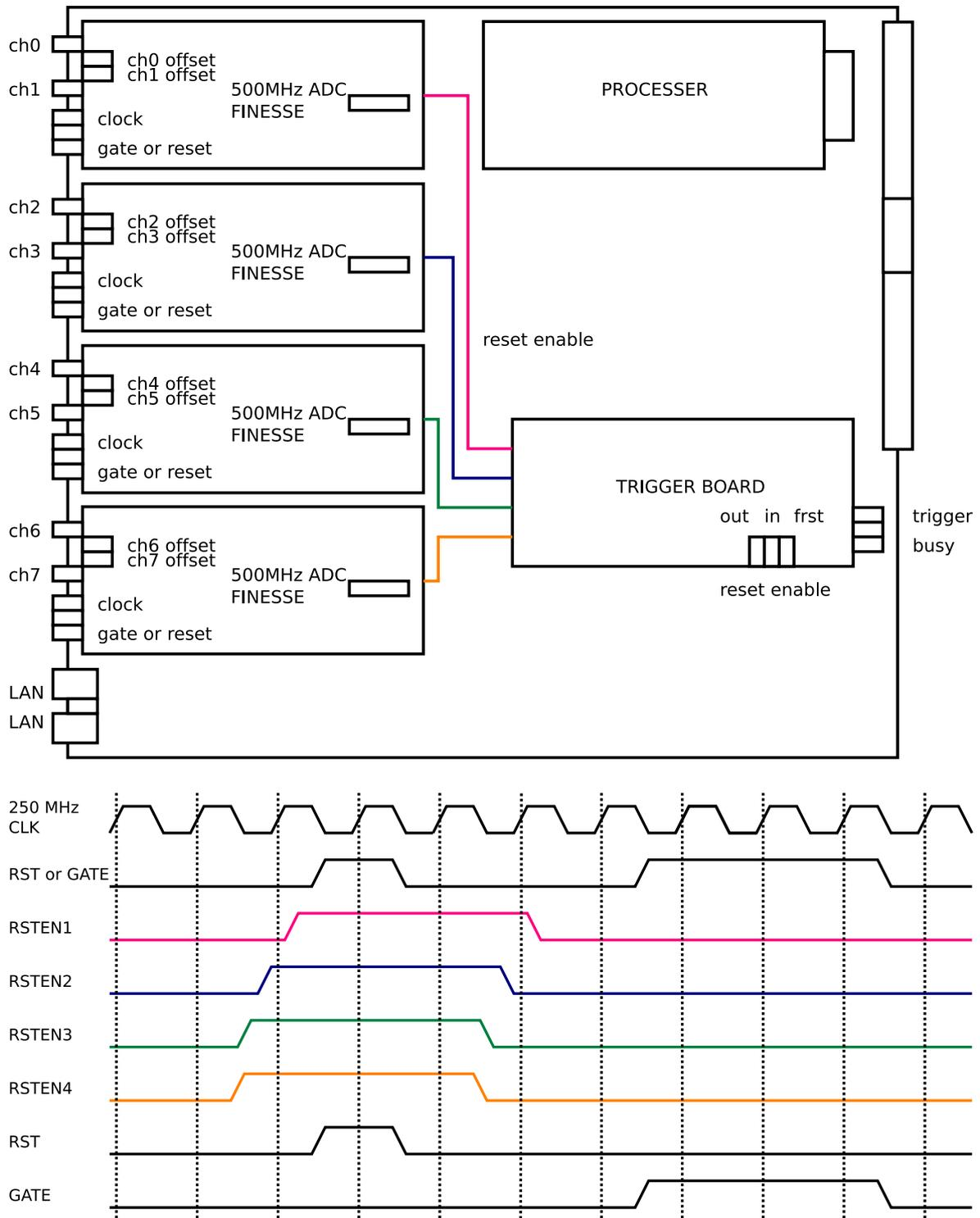
Figure 3.27: Timing chart of the reset from gate input AND the reset enable from the trigger card
