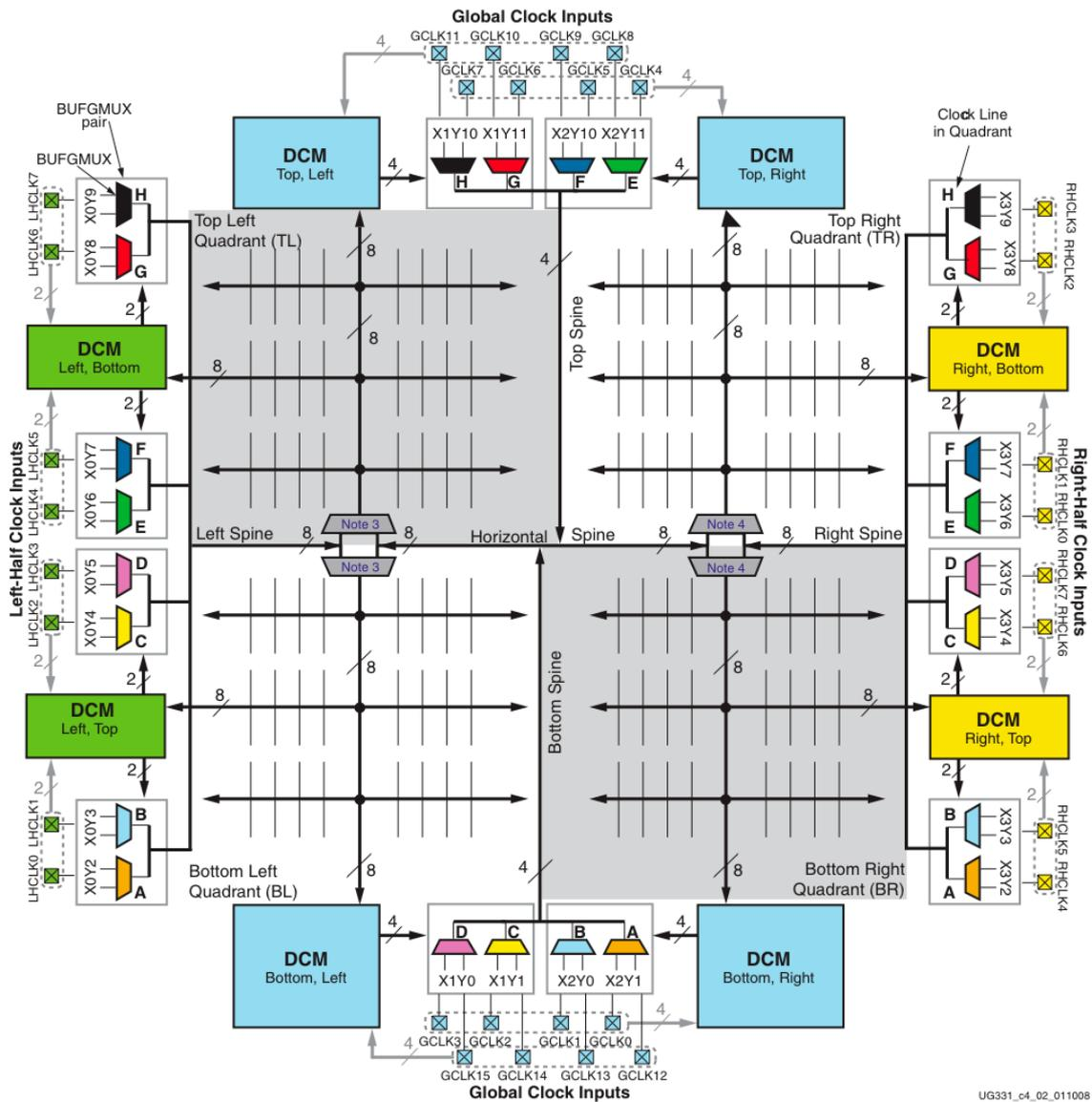
Figure 3.10: Diagram of signal lines and modules for clocks of Xilinx FPGA. Hardware DCM and MUX are located on near the edges of FPGA. Global clock line is also located over a FPGA.
