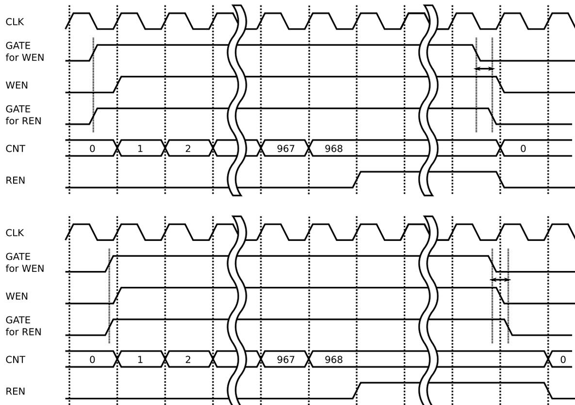
Figure 3.19: Timing chart of gate (GATE), write enable (WEN), and read enable (REN) signals latched by the same clock timing. GATE distributes the internal gate signals for WEN and for REN (GATEWEN and GATEREN). The timing that GATEWEN and GATEREN arrive at the modules can be different. FPGA sends WEN to FIFOs while the counter (CNT) stops sending REN to FIFOs.
