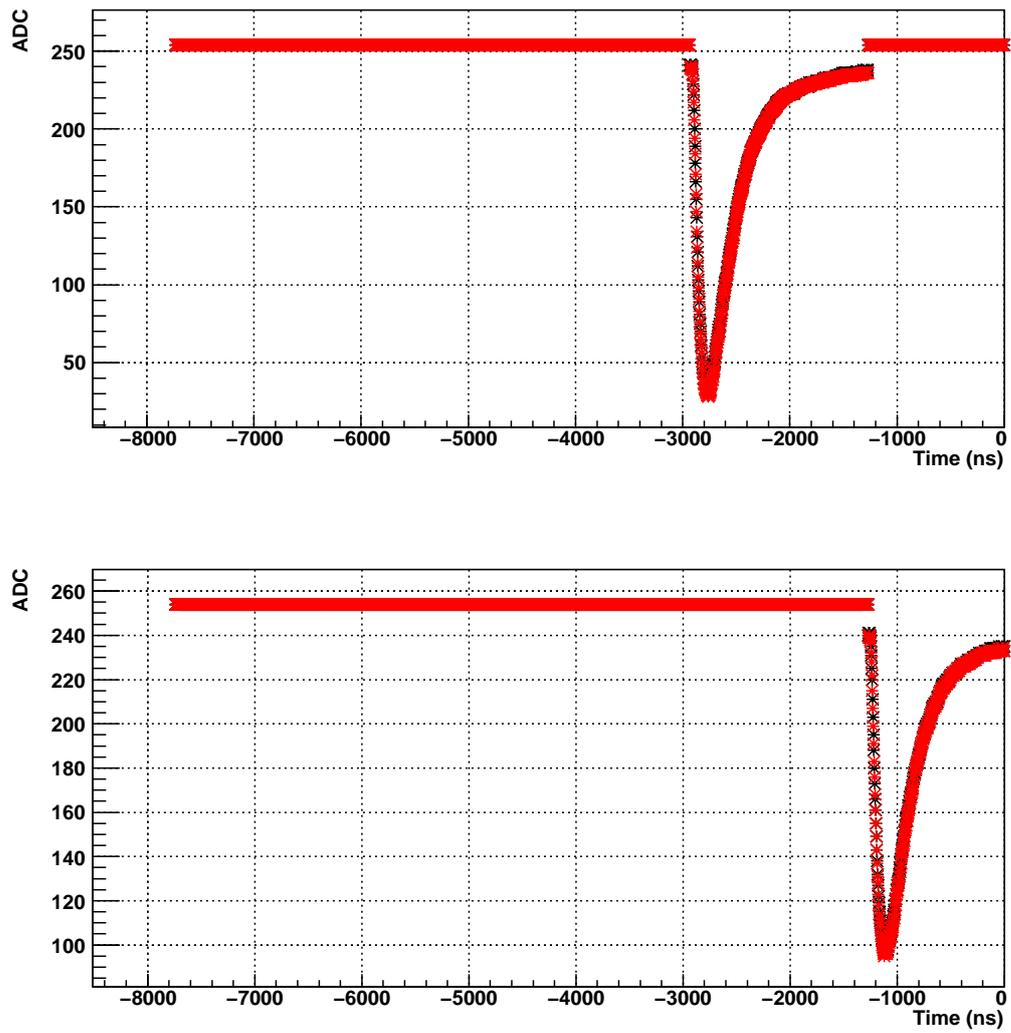
Figure 4.7: Waveforms of 1st COPPER with level 1 trigger, with level 0 + 1 trigger.
