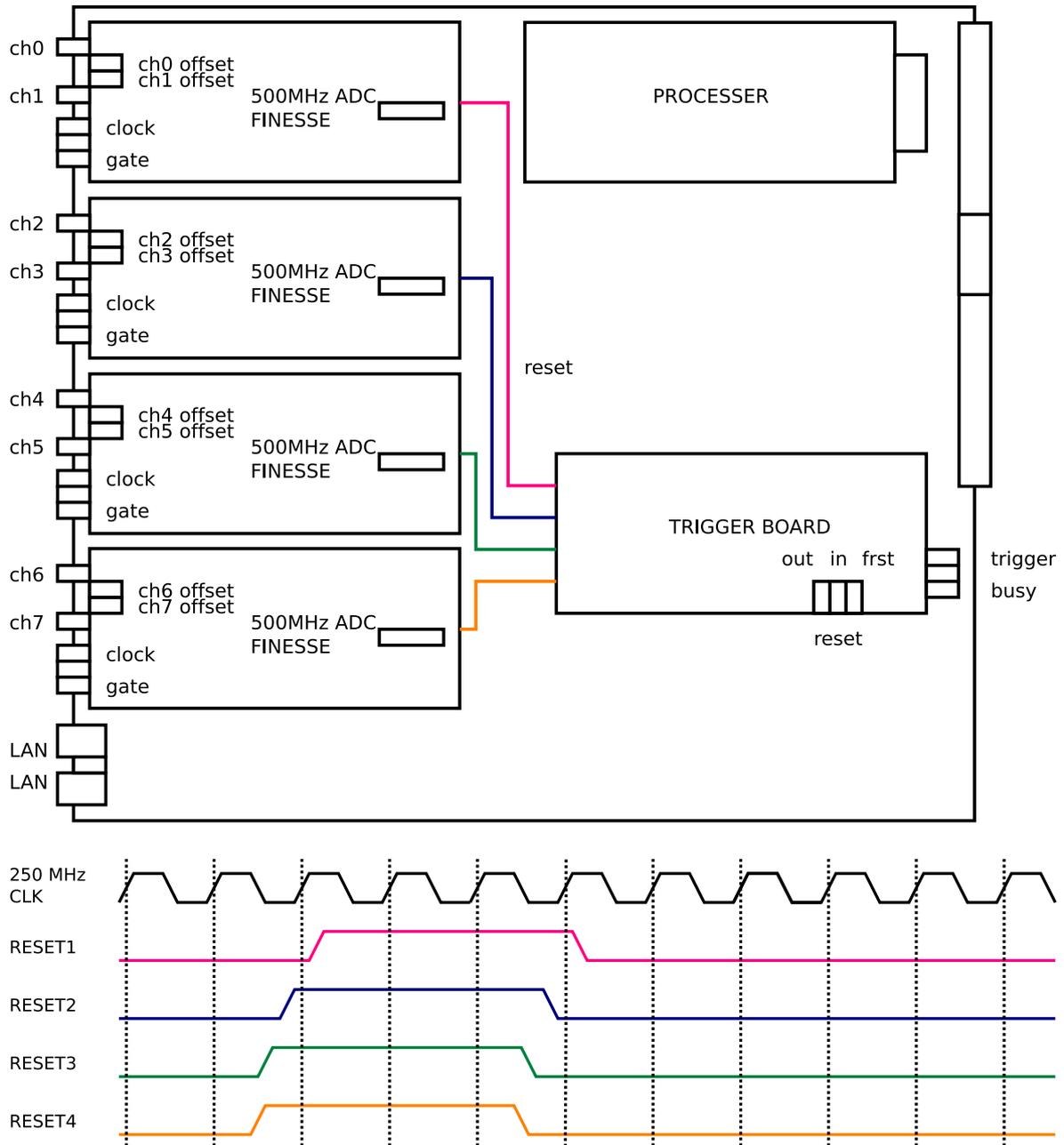
Figure 3.23: Schematics and diagram of the reset lines with different length. The different length allows the time of arrival at FINESSEs cross a clock timing.
