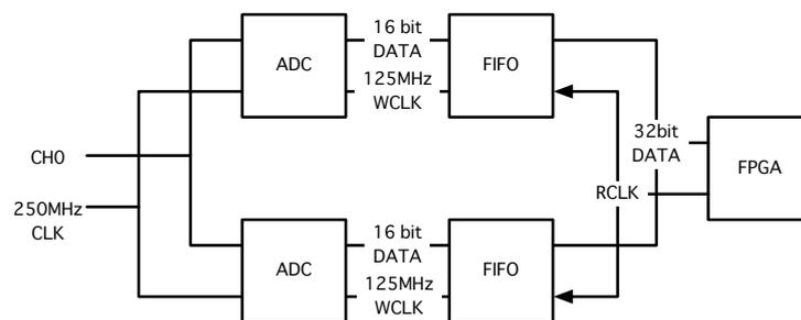
Figure 3.2: Schematics of one channel data from two ADCs and two FIFOs.
