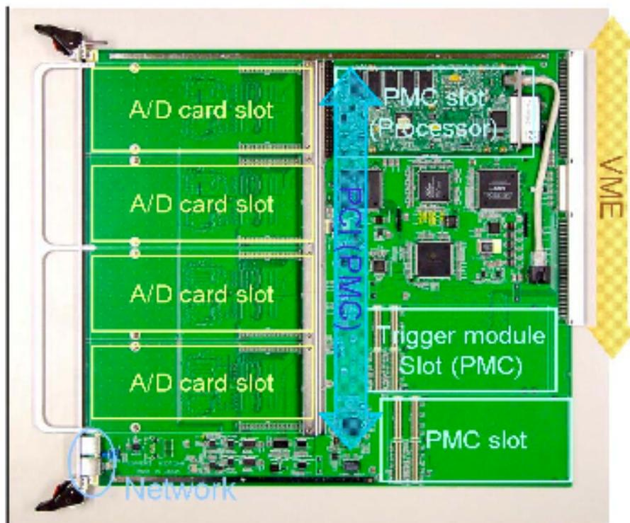
Figure 2.1: The layout of the COPPER mother board.
