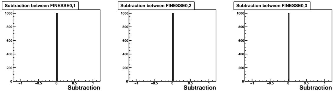
Figure 4.12: Difference of timestamps between four FINESSES. No difference is detected.
