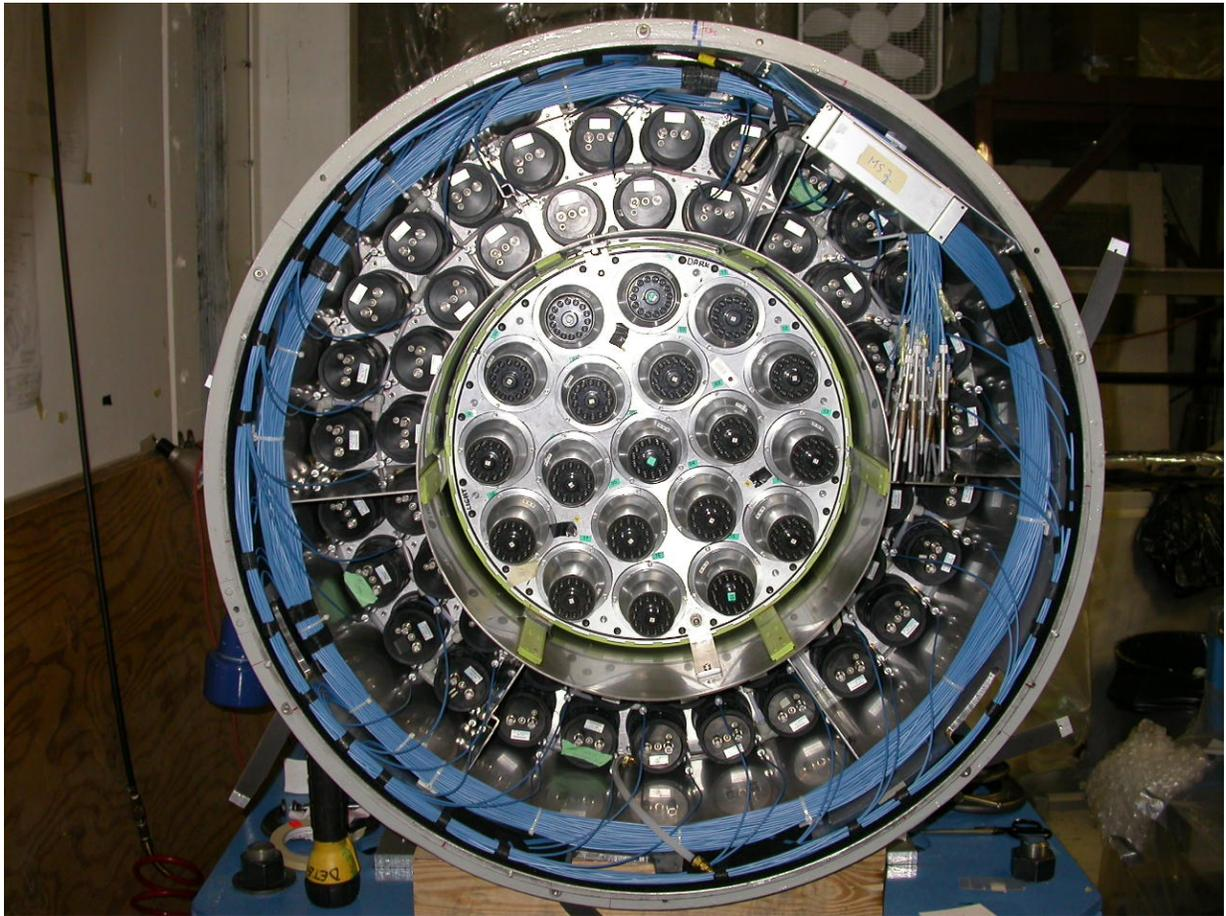
Figure 1.2: The PIENU calorimeter is comprised by a large NaI(Tl) crystal surrounded by 97 CsI crystals arranged in two rings.
