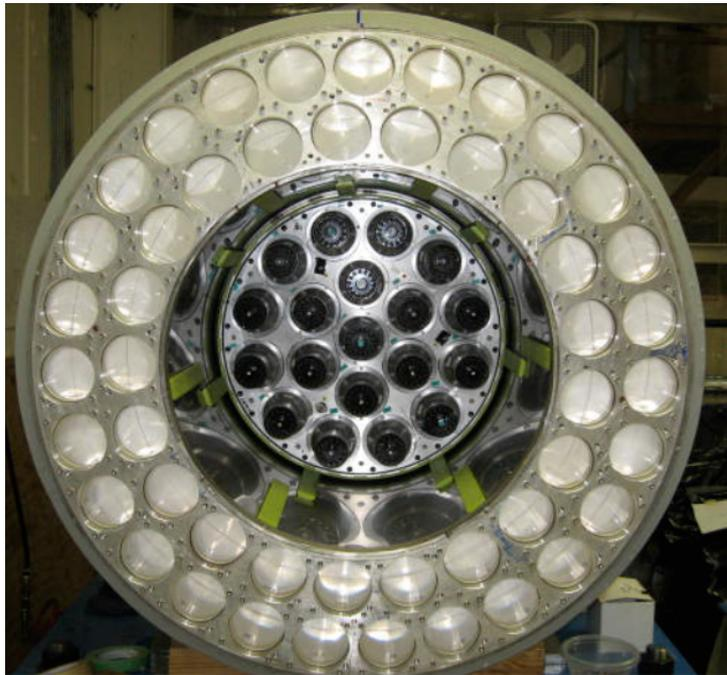
Figure 3.15: Picture of whole calorimeter consisted by NaI and 97 CsI crystals [3].
