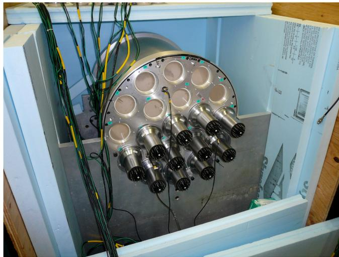
Figure 3.9: The BINA detector on the test bench, with some of its PMTs in place.
