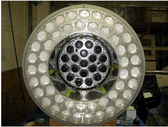
Figure 3.10: BINA and the two CsI rings, with all the BINA PMTs in place.
